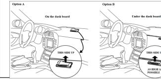
Connect the GPS antenna and wiring harness connector to the GPS Sniper unit. GPS antenna must be positioned horizontally and can not be shielded by any metal parts from above.
